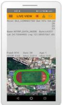
BLERTK Apps for iOS and Android are available for configuring GR-9028 and GR-9029. This allows smartphones, tablets, notebooks, and other BLE-enabled devices to communicate seamlessly with GR-9028 and GR-9029.
