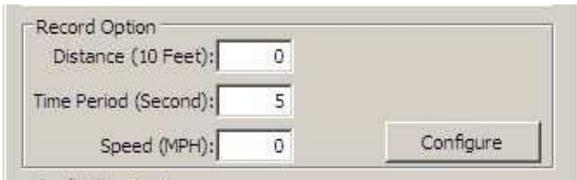
**Distance (Meter):** (0~20000) Log the position data by checking if the distance between this and previous point exceeds this value. For imperial unit only, the entered value is multiplied by 10 as the final distance setting.
