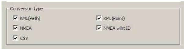
**KML (Path):** Google Earth format that displays positions with continuous path. Following picture is an example.
