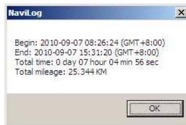
The mileage summary is the result from the first (start) to the last (stop) logged data. Please note that the **Begin** time and **End** time depend on the time zone setting. The unit of **Total mileage** also depends on the Imperial or Metric unit is set. If KM/h is selected, it is KM. If MPH is selected, it is Mile.
