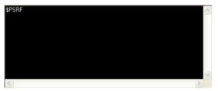
For example, following commands will disable GGA, GSA, GSV, VTG output and set RMC to output every minute. \$PSRF103,00,00,00,01\*24 (Disable GGA output) \$PSRF103,02,00,00,01\*26 (Disable GSA output) \$PSRF103,03,00,00,01\*27 (Disable GSV output) \$PSRF103,05,00,00,01\*21 (Disable VTG output) \$PSRF103,04,00,60,01\*26 (RMC output @ 1/60Hz)
