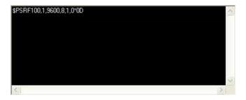
and the output stops since the baud rate has been changed. Please close and reopen with new baud rate. Following is a summary for different baud rate settings:
